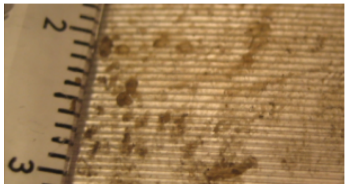
Figure 5: Flake of plastic coating from outer lip of rim.
