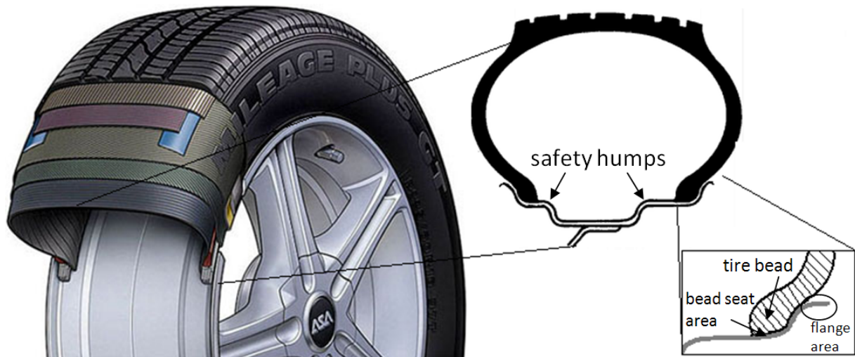
Figure 1: Anatomy of a wheel-tire assembly. The tire is marked solid black. The cylindrical portion of the wheel, the rim, is marked in grey. Air is enclosed between the tire and rim; air pressure within the chamber is maintained by the seal formed between the tire bead and the bead seat. Image modified from [1-2].
