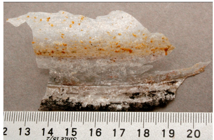
Figure 4: Flake of plastic coating from outer lip of rim.
