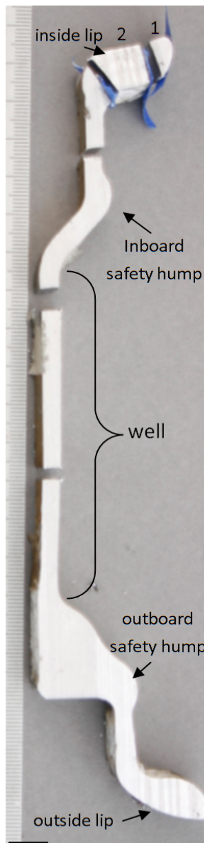
Figure 3: Terms used to reference parts of a rim. Scale bar = 1 cm. Labels 1 and 2 refer to samples used for cross-section surface examination.
